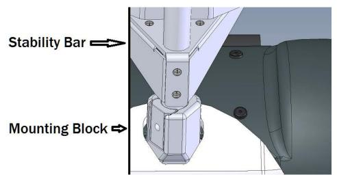
3. Replace the attachment screw on the mounting block and finger tighten. Once finger tight, use the Allen key to tighten the bolt down securely to 30 Nm (22 foot-pound). Ensure that the locking washer and flat washer are installed in the same orientation as when removed.
