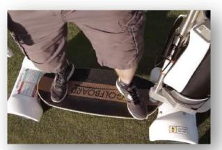
Shift your body weight from one side of the board to the other in order to turn. As weight is increasingly applied to one edge of the board, the wheels pivot causing the board to turn. The stability bar can also be pushed or pulled right or left to enhance turning ability. However, you should primarily use the shifting of your weight from toes to heels as the principal way to steer a GolfBoard.
